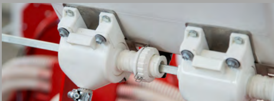
With an increasing amount of insects killing plants during growing and an increased need of microfertilizer, increases the need of microgranule applicators. Vegetable planters can be equipped with microgranule applicators. The hoppers are made of special grade plastics and have a capacity of 35 litres. The hoppers supply 2 planting units.
