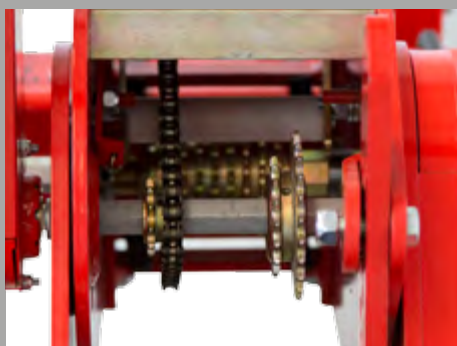
Through multi-speed transmission, is possible to sow in 32 speed positions.
